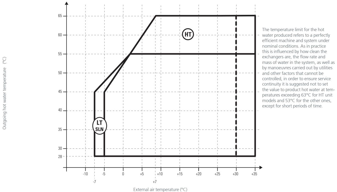
THE THERMAL GRADIENT OF THE WATER FOR ALL VERSIONS MUST BE BETWEEN: min:4 °C max: 7°C
